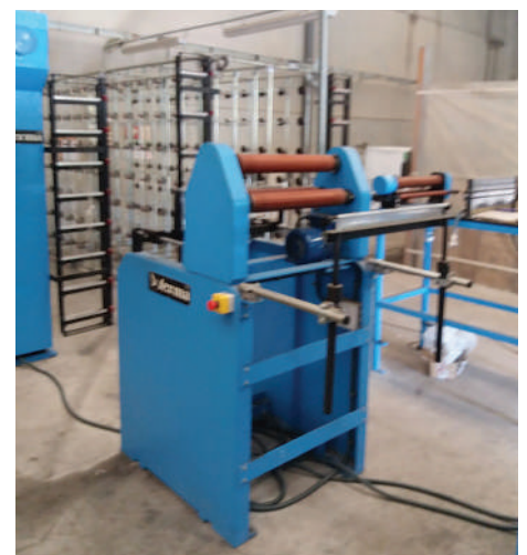
Pre-estiraje positivo Positive pre-stretching
