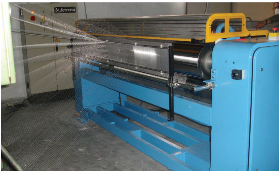
Parte trasera con 3 rodillos de alimentación Backside group with 3 self-powered rollers
