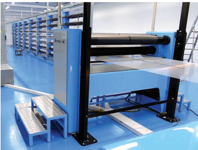
Pre-estiraje situado entre fileta y urdidor Pre-stretching device fitted between creel and warping head
