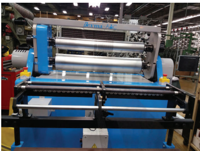
Parte trasera con rodillos auto-alimentados Backside group with self-powered rollers
