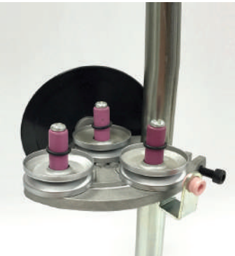
Tensor 3 pivotes desde 0 hasta 3000 dtex Tensioner with 0 pins from 0 to 3000 dtex
