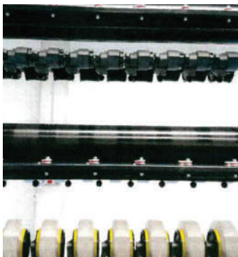
Guía hilos elastómero CGE. Threads guide for elastomeric yarn CGE.
