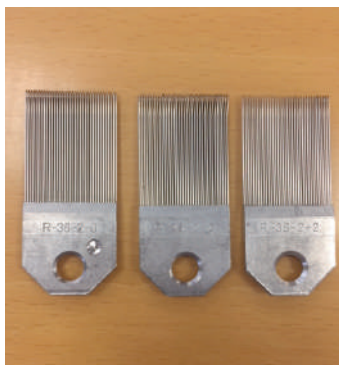
Plomos urdidor (1"). Comb leads for Warper (1").
